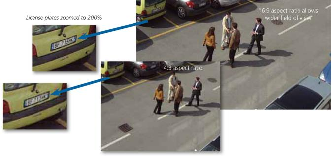
A standard D1 resolution image overlaid on a MegaPX 720p MiniDome image (1280x720)
